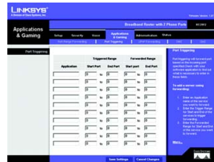
Figure 5-19: Applications & Gaming Tab - Port Triggering
