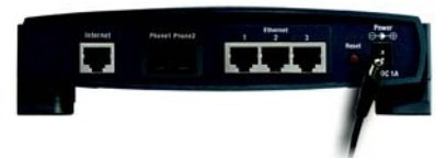
Figure 4-4: Connect the Power
