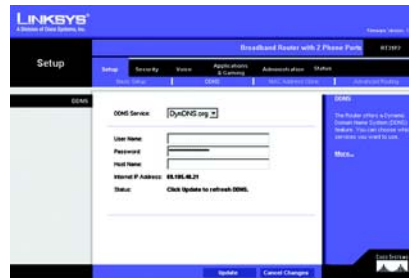
Figure 5-9: Setup Tab - DDNS (DynDNS.org)
