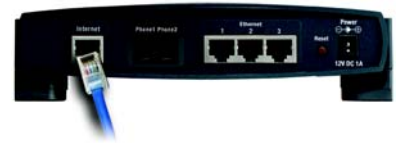
Figure 4-3: Connect the Modem
